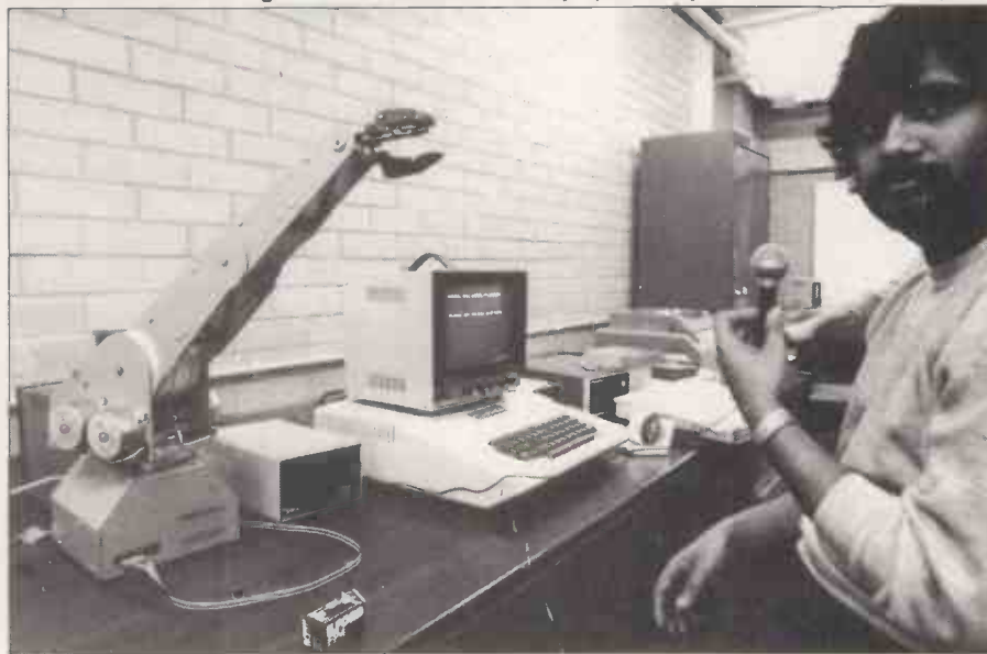
Prakash Sinha directing an Armdroid robot arm by speech input
